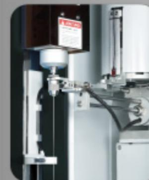
The unique characteristic of Ram type structure offers an outstanding Z axis stroke up to 700 mm. Optional 700 mm. electrode tube is available
