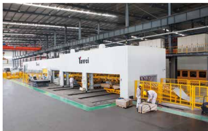
Cut to Length Line With Oscillating Shear
